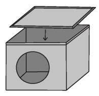
We recommend adding a Plenum to improve the process of Indoor Air Handler installation and efficiency, as it is easily mounted to the unit.
